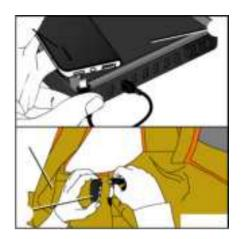
Insert the mobile warning unit (1) into the designated pocket (3) with the rear side facing outwards and upwards and connect it to the USB cable (4).
