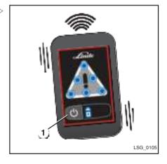
The LEDs light up briefly. A signal tone sounds. The Distance Beeper vibrates briefly and shuts down
