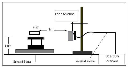
(B) Radiated Emission Test-Up Frequency 30MHz~1GHz
