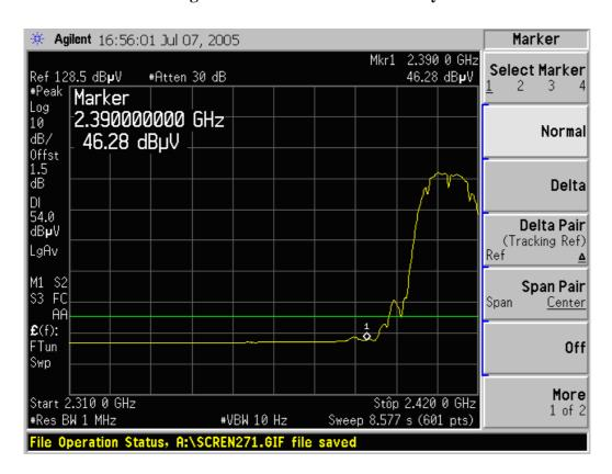
Detector mode: Peak Polarity: Horizontal
