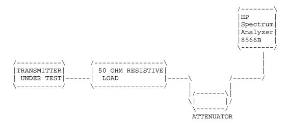
NAME OF TEST: SPURIOUS EMISSIONS AT ANTENNA TERMINALS
