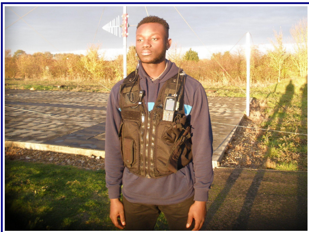
Photo 8: SC2120 Lapel-worn with 2-WK cable parallel to antenna
