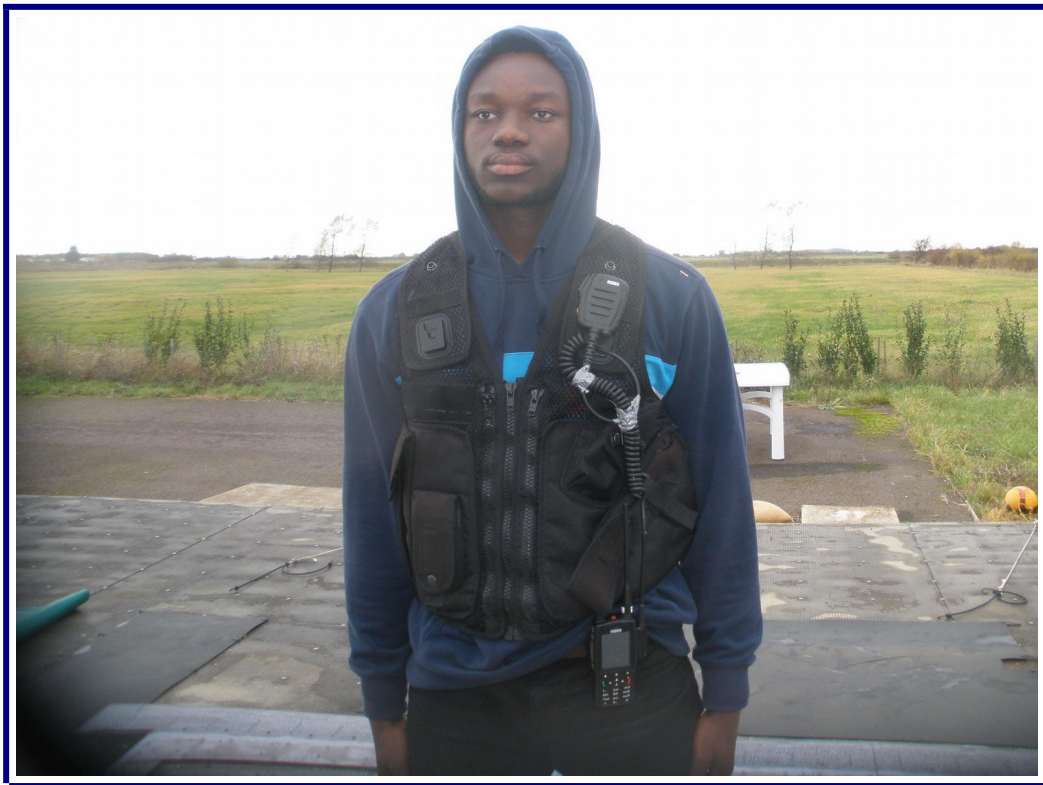
Photo 7: SC2124 Belt-worn with B-RSM cable parallel to antenna
