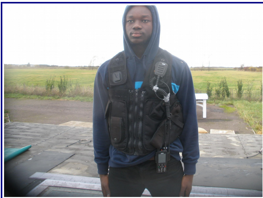
Photo 6: SC2120 Belt-worn with B-RSM cable parallel to antenna
