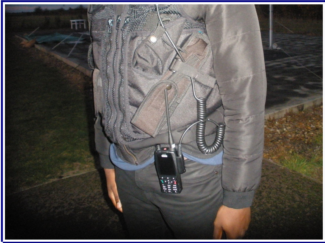
Photo 9: SC2120 Belt-worn with B-RSM cable free hanging
