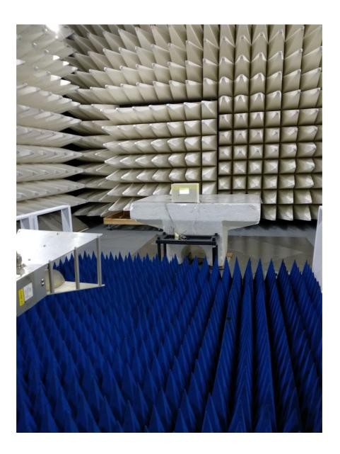
$\label{eq:Photograph No.6} Photograph No.6 \\ Spurious emissions measurement setup in the anechoic chamber in 18 – 27 GHz$
