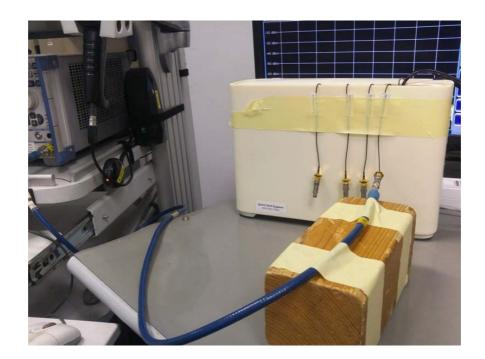
Photograph No.3 Spurious emissions measurement setup in the anechoic chamber, EUT close view
