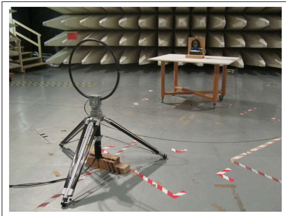
Photograph A1-2: Radiated emissions 9 kHz – 30 MHz at 3 m distance at SAC and Occupied Bandwidth
