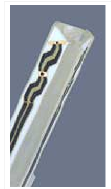
Inside view of ET3DV6 E-field Probe
