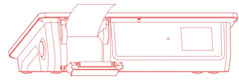
After printing, tear the paper upwards.
