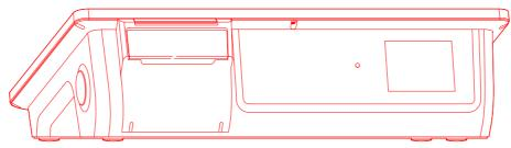
Insert the thermal paper and pull out part of it outside the paper exit of the printer, then close the paper compartment cover;
