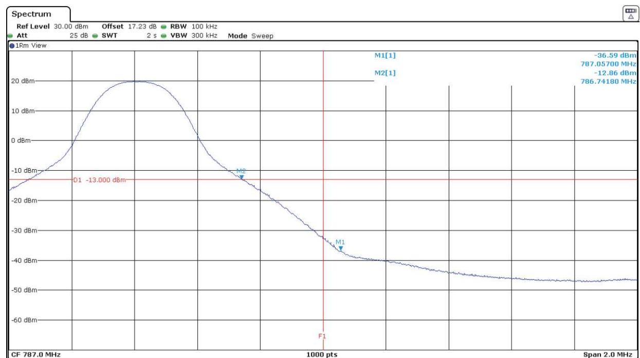
LTE Band 13. QPSK MODULATION. BW=10 MHz. RB=All. Offset=0. Lowest and Highest Block Edges:
