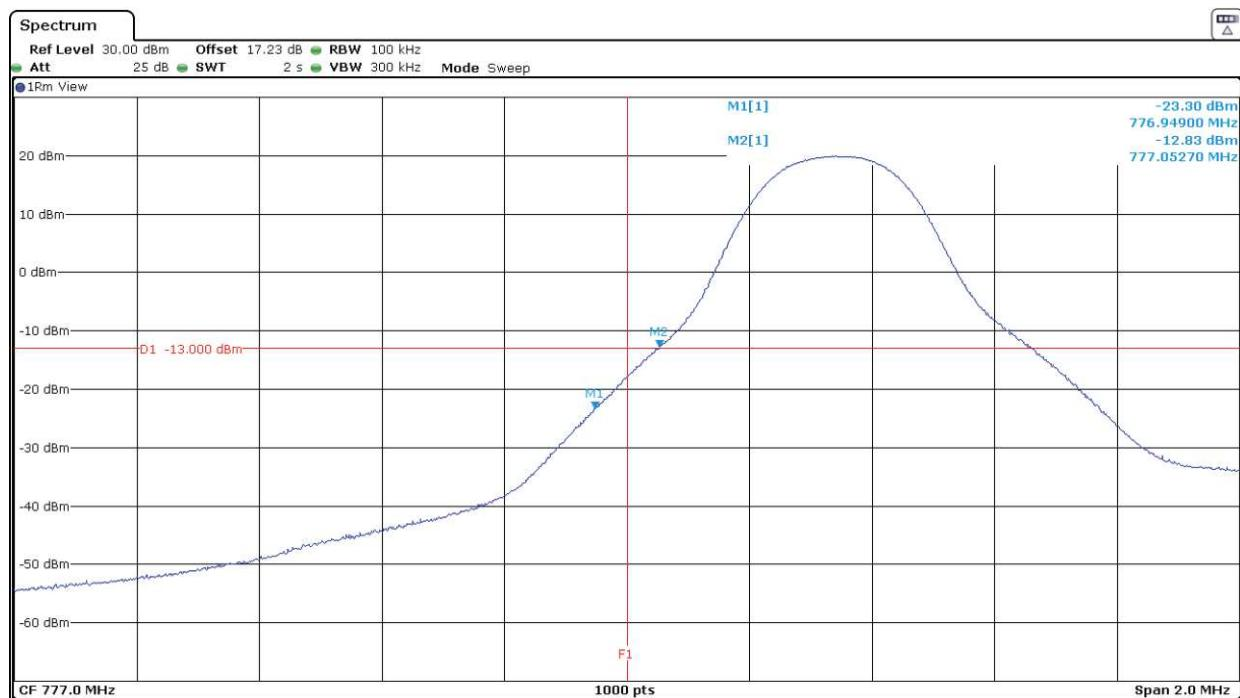
LTE Band 13. QPSK MODULATION. BW=5 MHz. RB=1. Offset=Max. Highest Block Edge:
