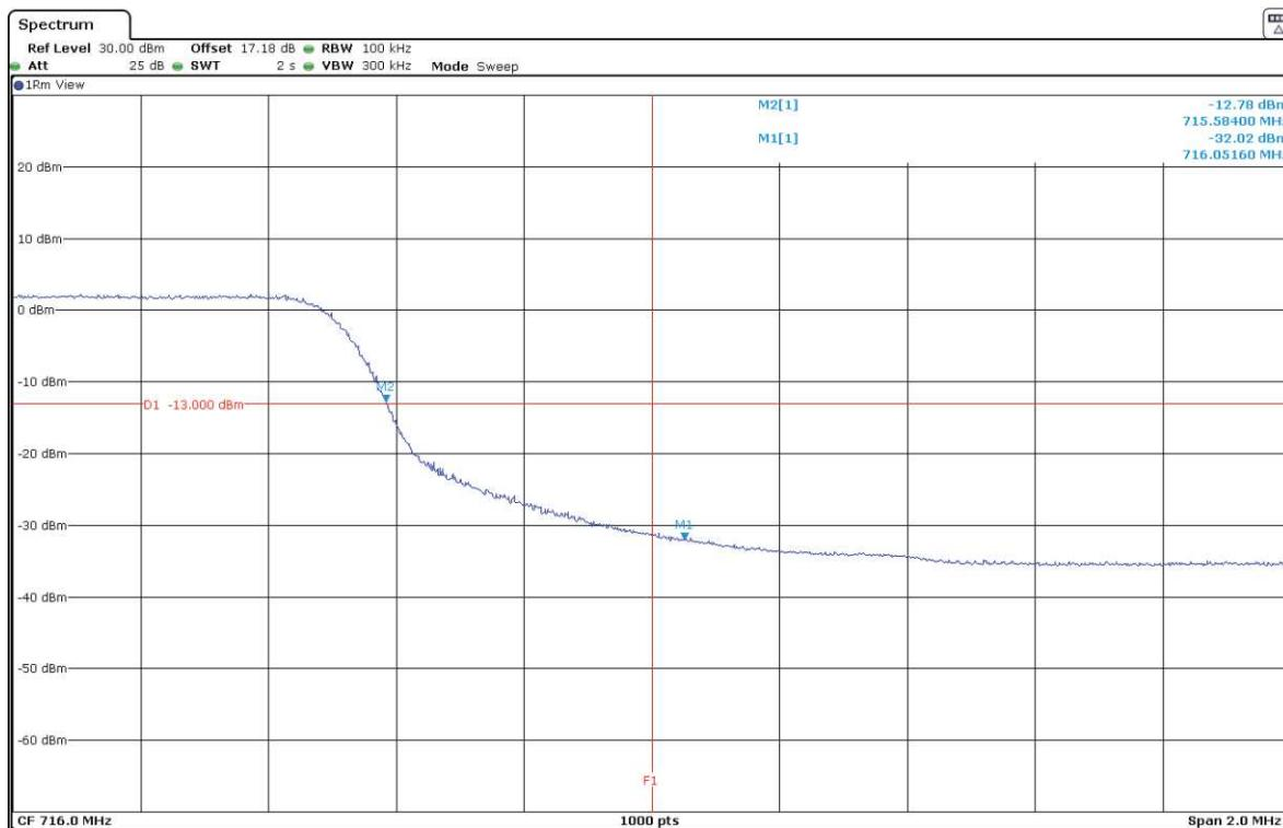
LTE Band 13. QPSK MODULATION. BW=5 MHz. RB=1. Offset=0. Lowest Block Edge:
