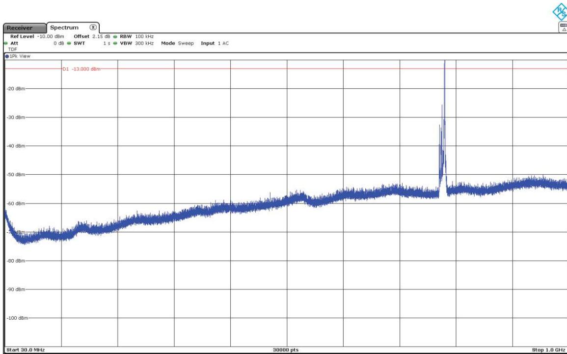
The peak above the limit is the LTE Band 13 carrier frequency (782 MHz).
