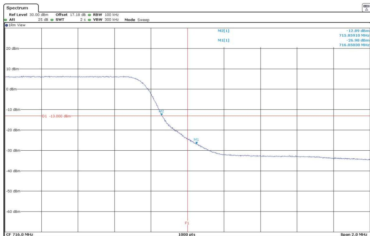
LTE Band 12. QPSK MODULATION. BW=10 MHz. RB=1. Offset=0. Lowest Block Edge:
