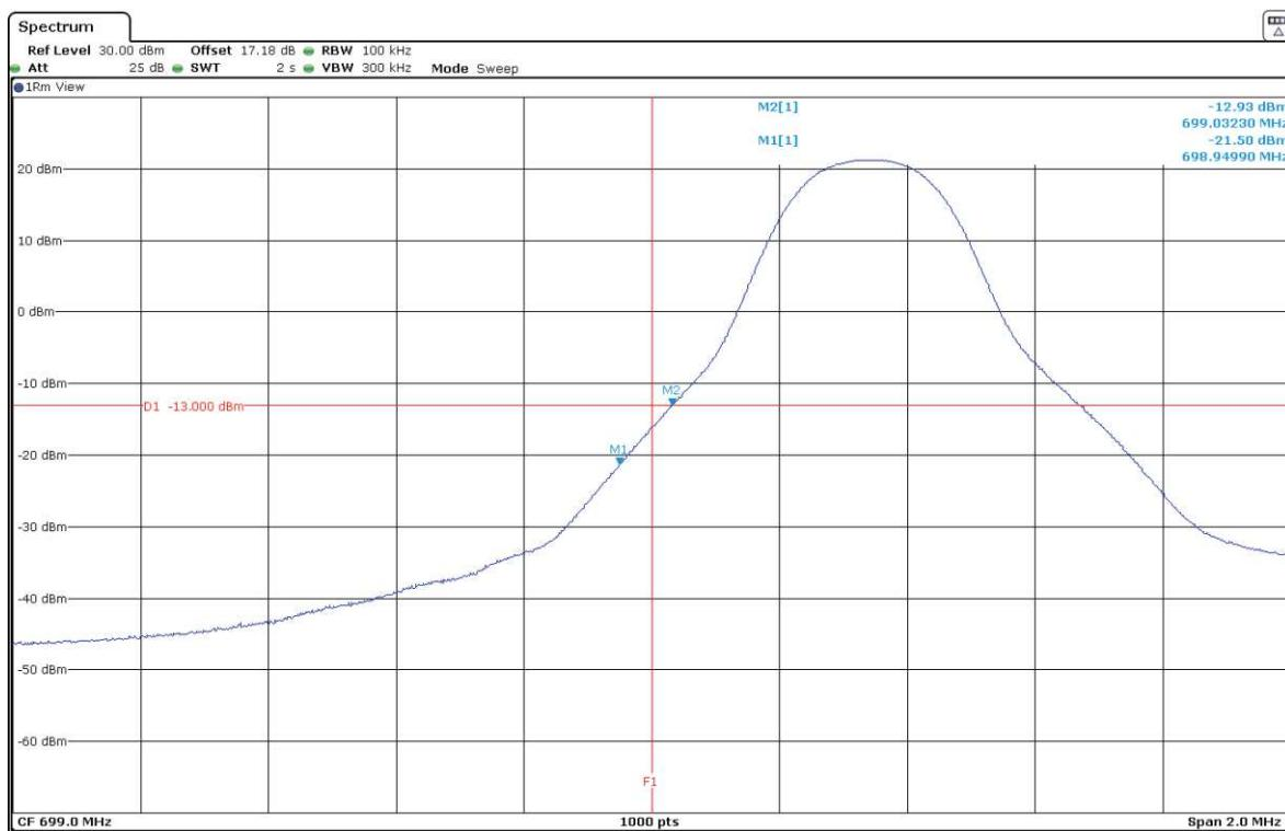
LTE Band 12. QPSK MODULATION. BW=5 MHz. RB=1. Offset=Max. Highest Block Edge:
