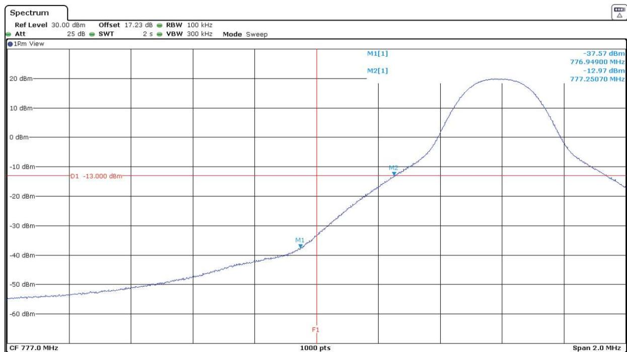
LTE Band 13. QPSK MODULATION. BW=10 MHz. RB=1. Offset=Max. Highest Block Edge:
