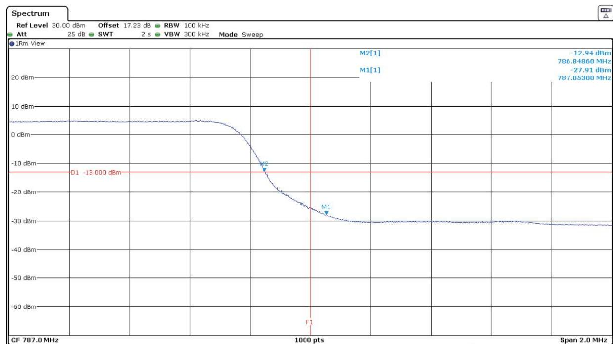
LTE Band 13. QPSK MODULATION. BW=10 MHz. RB=1. Offset=0. Lowest Block Edge:
