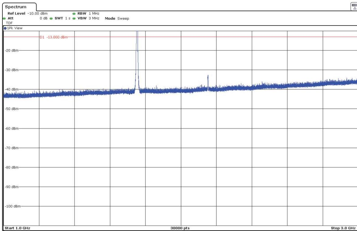
The peak above the limit is the 3G Band IV carrier frequency (1752.6 MHz).
