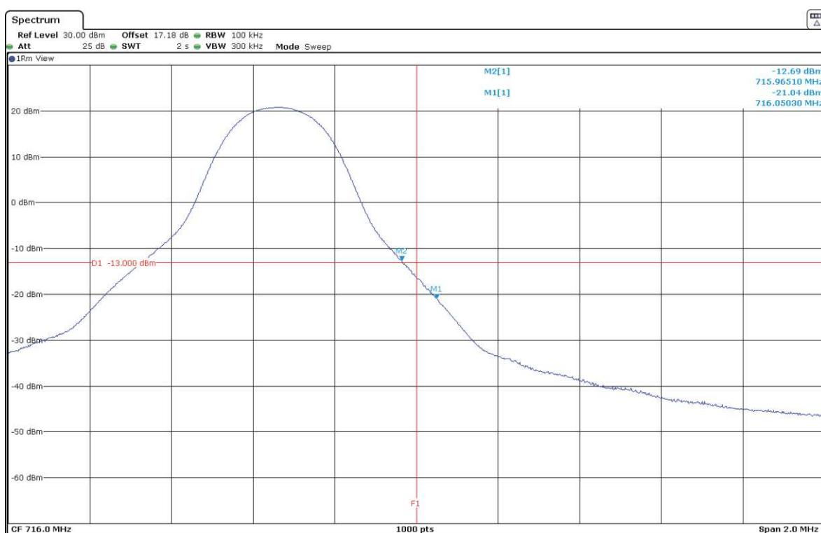
LTE Band 12. QPSK MODULATION. BW=5 MHz. RB=All. Offset=0. Lowest and Highest Block Edges:
