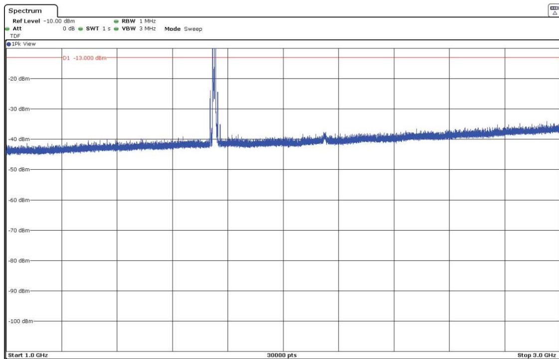
The peak above the limit is the LTE Band 4 carrier frequency (1750 MHz).
