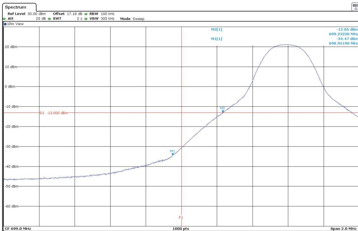
LTE Band 12. QPSK MODULATION. BW=10 MHz. RB=1. Offset=Max. Highest Block Edge:
