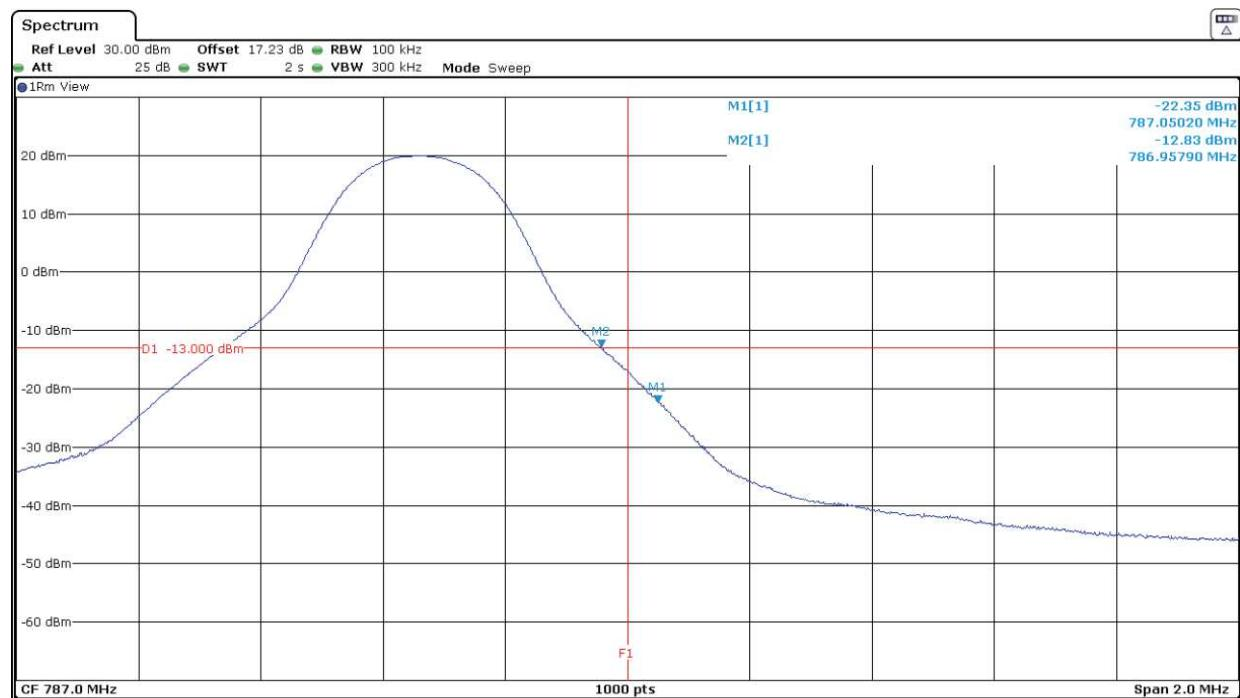
LTE Band 13. QPSK MODULATION. BW=5 MHz. RB=All. Offset=0. Lowest and Highest Block Edges:
