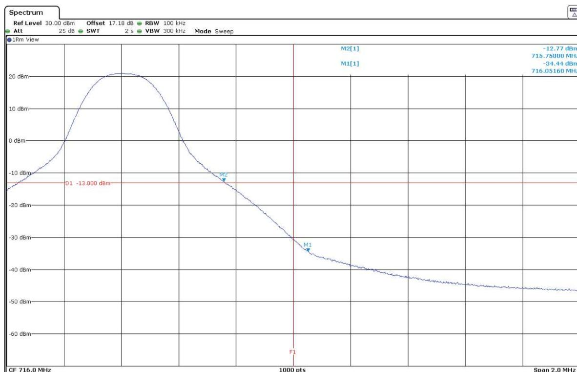
LTE Band 12. QPSK MODULATION. BW=10 MHz. RB=All. Offset=0. Lowest and Highest Block Edges:
