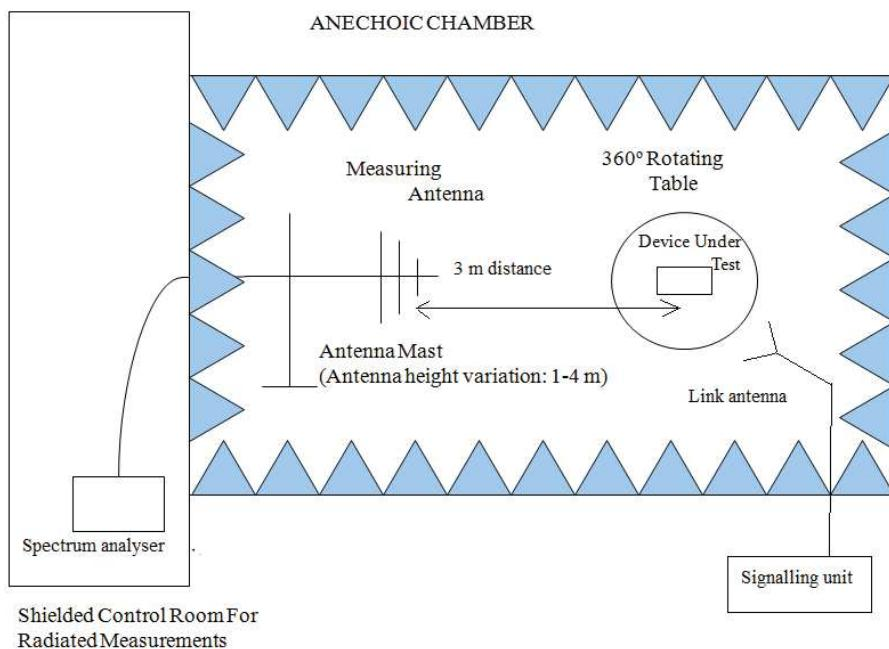
Radiated measurements above 1 GHz.
