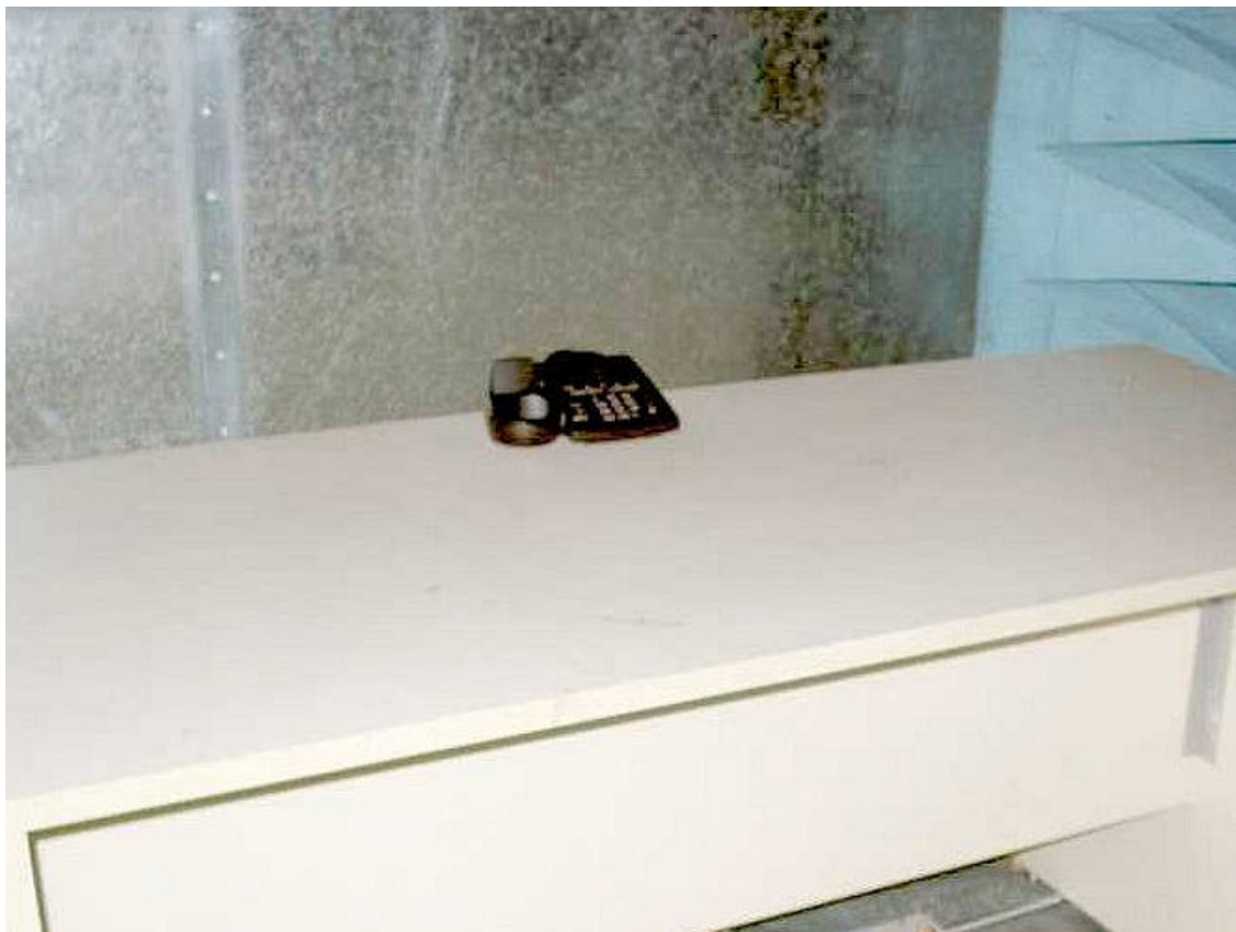
Testing Conducted Emissions on Power Lines Base unit connected to LISN Frequency range: 450 kHz – 30 MHz
