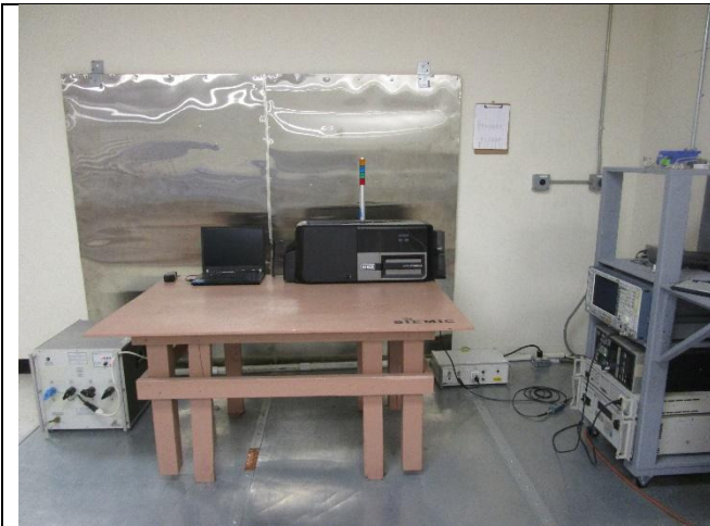
AC Line Conducted Emissions– Front View
