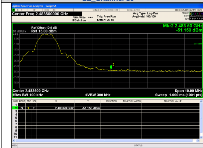
Out Of Band Emission LE_Channel 39
