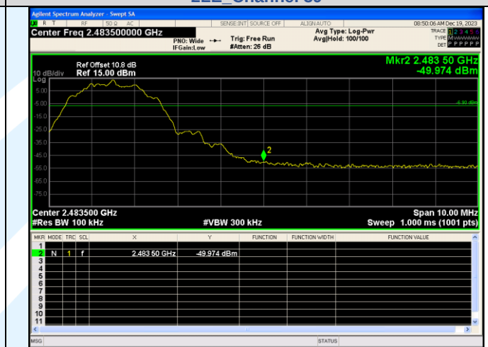
Out Of Band Emission 2LE_Channel 39
