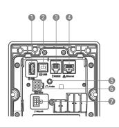
USB - host USB-device RS232 Ethernet Audio MDB Microfit
