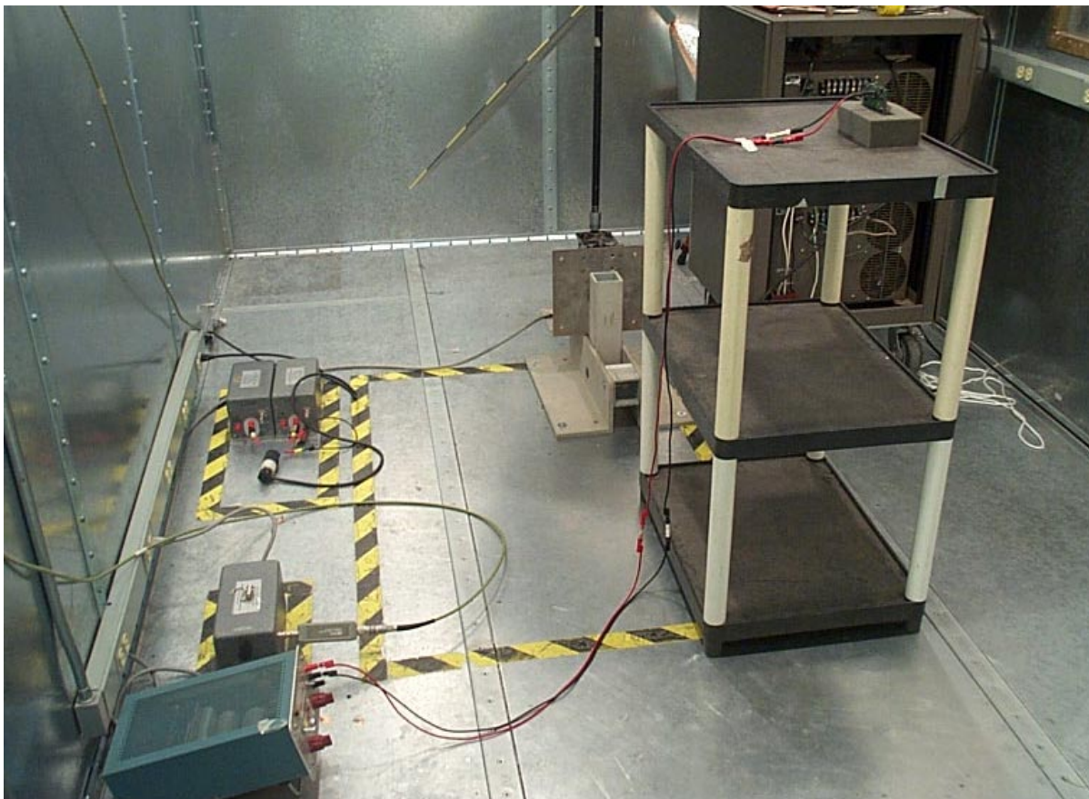
FIGURE 6A - 1 CAD+ AC CONDUCTED EMISSIONS TEST SETUP
