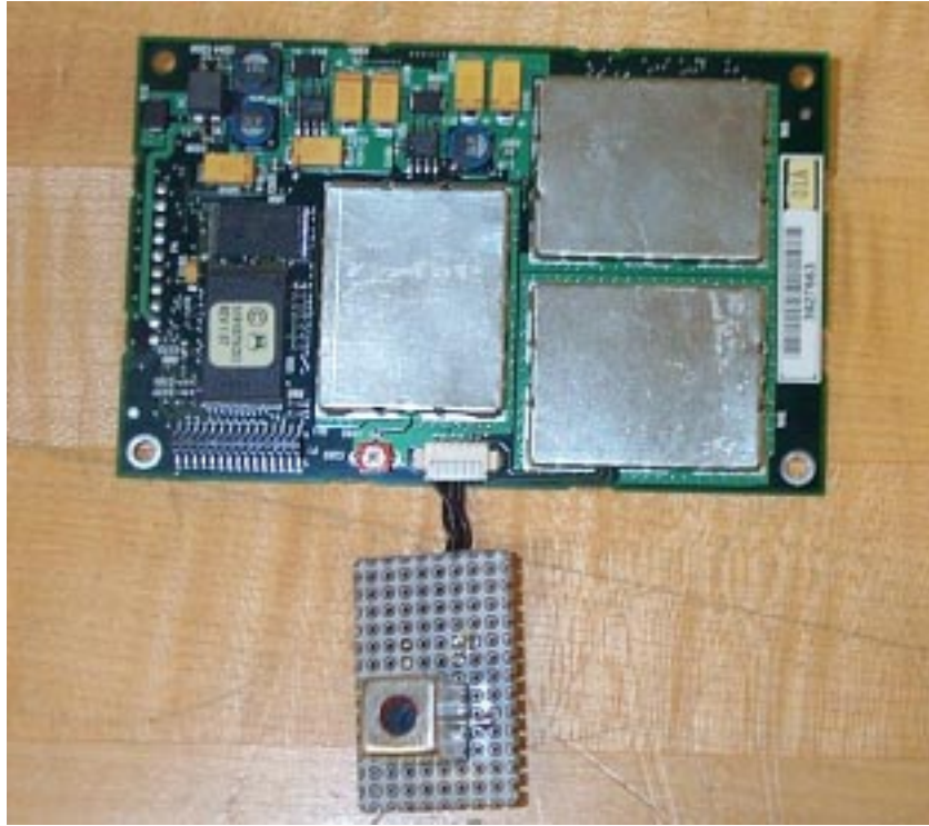
FIGURE 6A - 2 CAD+ with Antenna dummy load
