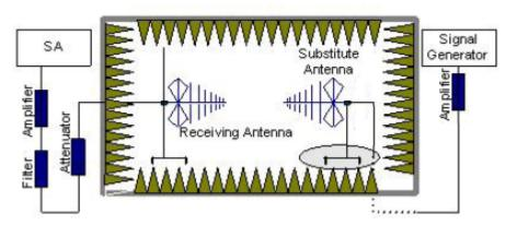
In the chamber, a substitution antenna for the frequency band of interest is placed at the reference point of the chamber. An RF Signal source for the frequency band of interest is connected to the substitution antenna with a cable that has been constructed to not interfere with the radiation pattern of the antenna. A power ( $P_{\text{Mea}}$ ) is applied to the input of the substitution antenna, and adjust the level of the signal generator output until the value of the
