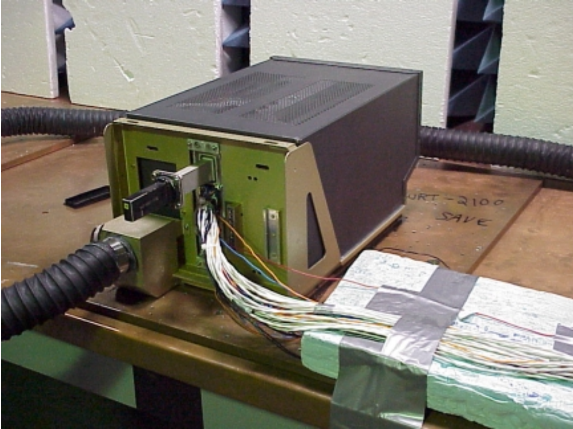
Figure 12-3. Radiated Emissions Setup - Per DO-160D and Boeing Requirements
