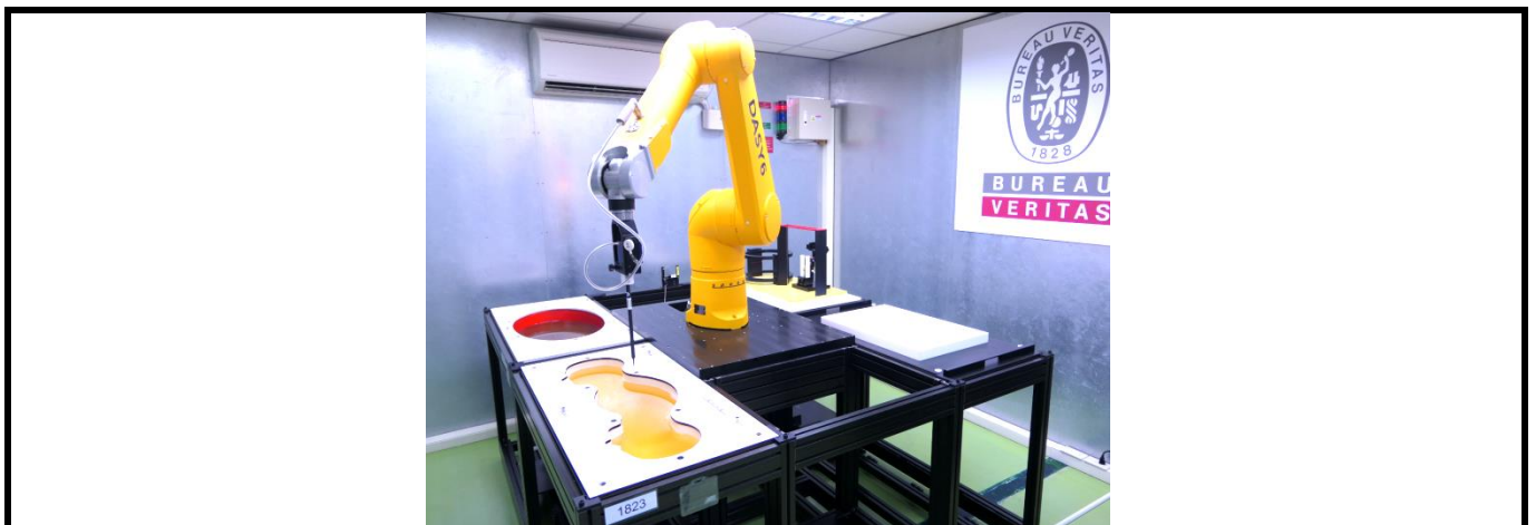
Fig-3.2 SPEAG DASY6 System
