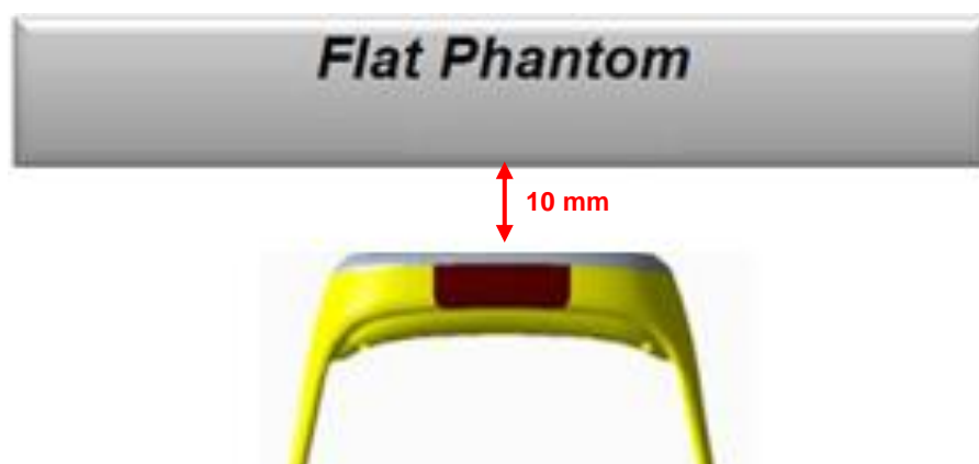
Fig-4.2 Illustration for Face Exposure Setup
