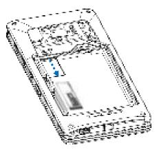
Place the Nano SIM and/or Micro SD/Nano SAM card into the carrier with contact side face down.
