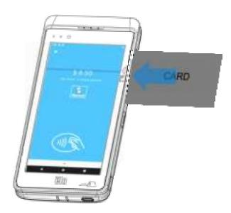
Bidirectional MSR capable of reading up to three tracks of data on ISO 7810/7811.
