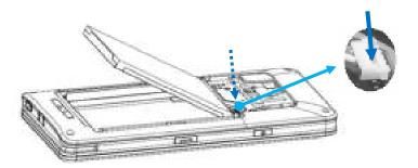
• Insert the battery into the compartment.
