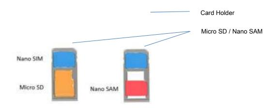
• Insert the carrier back into the Micro SD card compartment.
