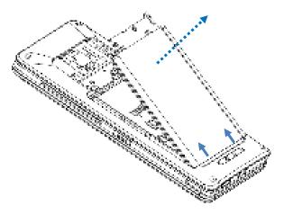
Push and lift up the metal shield of the battery using your finger.
