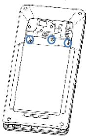
• Place the access point cover and snap into place to secure.
