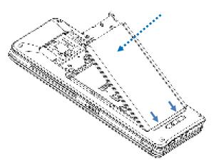
• Fasten the battery cover with 3 screws.
