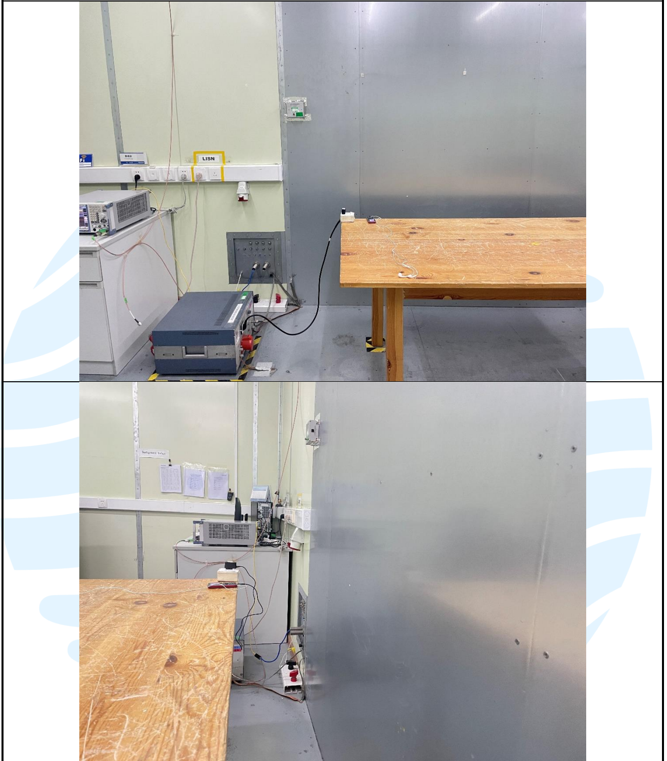
Conducted Emission Test Setup-3
