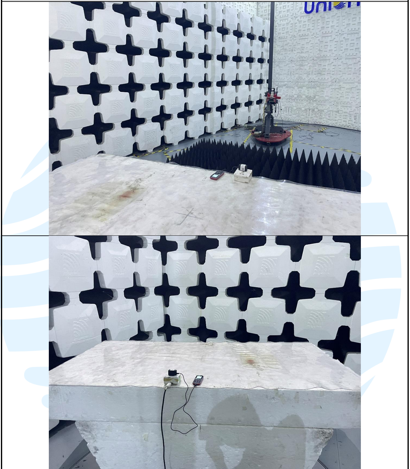
Radiated emission Test Setup-2 (Above 1 GHz)
