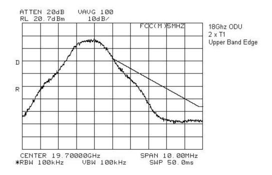
EQUIPMENT: Digital Microwave Radio, 18 GHz ODU
