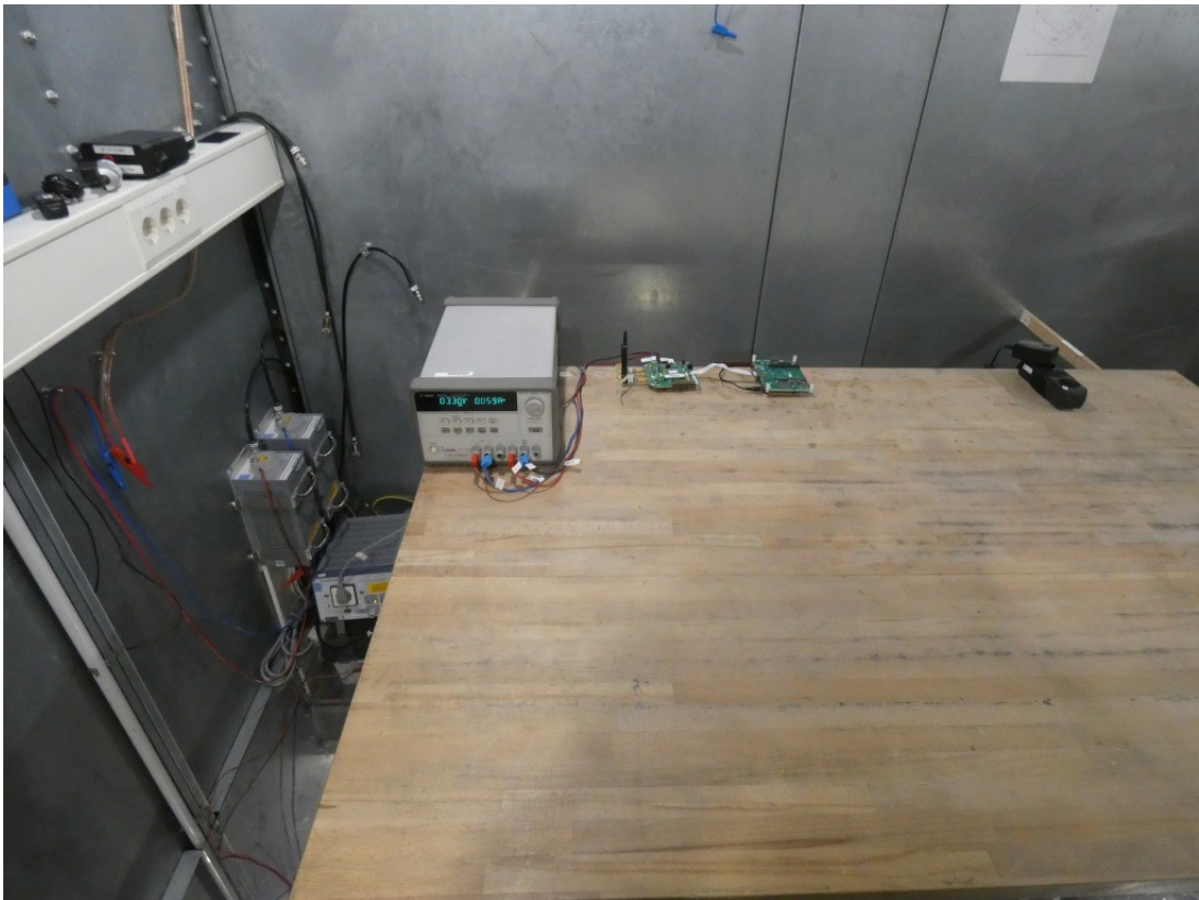
Photo 1: Test setup for conducted measurements below 30 MHz
