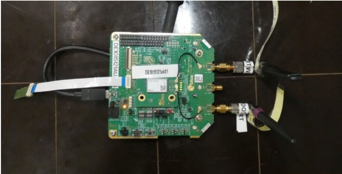
Photo 5: Test setup for radiated measurements EUT detail
