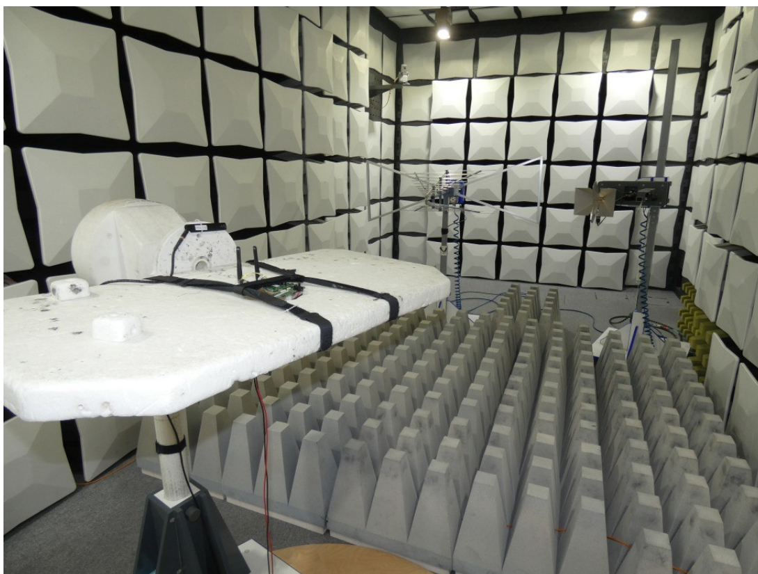
Photo 3: Test setup for radiated measurements above 1 GHz
