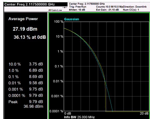
Channel: BOTTOM, Modulation: 256QAM, BW=15MHz, CCDF
