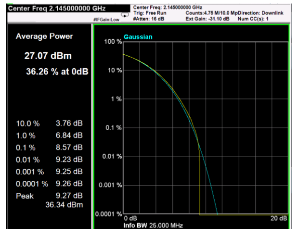
Channel: MIDDLE, Modulation: 16QAM, BW=20MHz, CCDF
