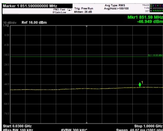
Channel: TOP, Modulation: 16QAM, BW=10MHz, Range: Lower
