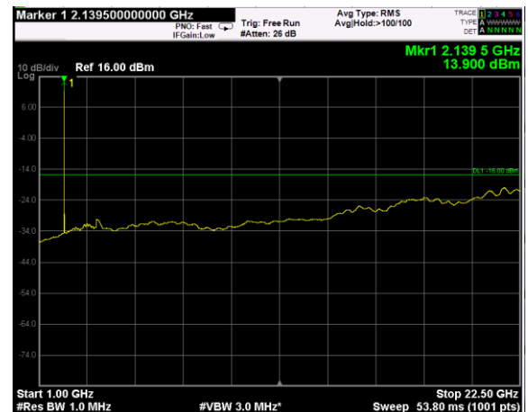
Channel: MIDDLE, Modulation: 256QAM, BW=5MHz, Range: Upper
