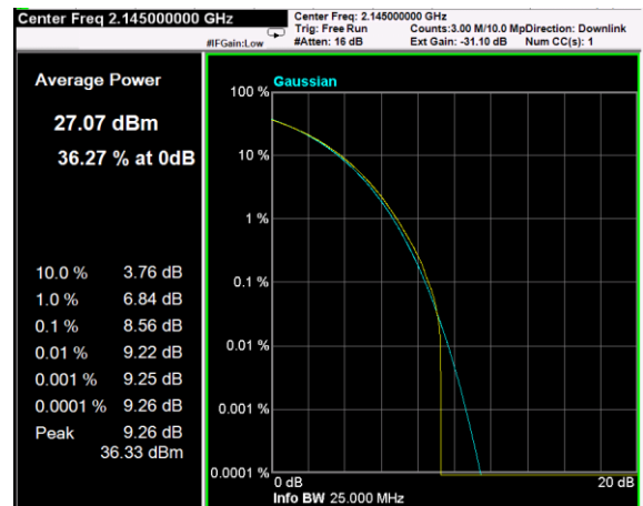
Channel: MIDDLE, Modulation: 256QAM, BW=20MHz, CCDF
