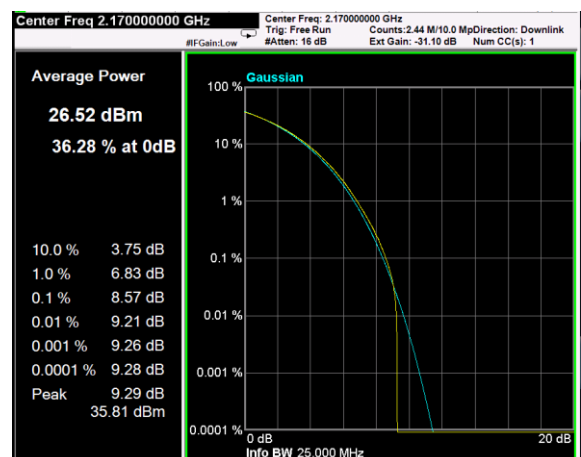
Channel: TOP, Modulation: 16QAM, BW=20MHz, CCDF
