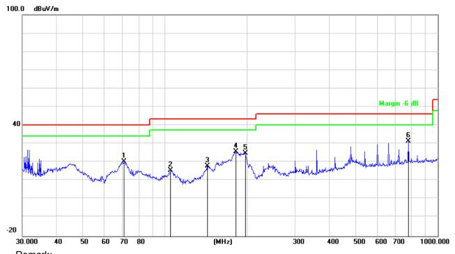
Remark: Factor = Antenna Factor + Cable Loss - Amplifier.
