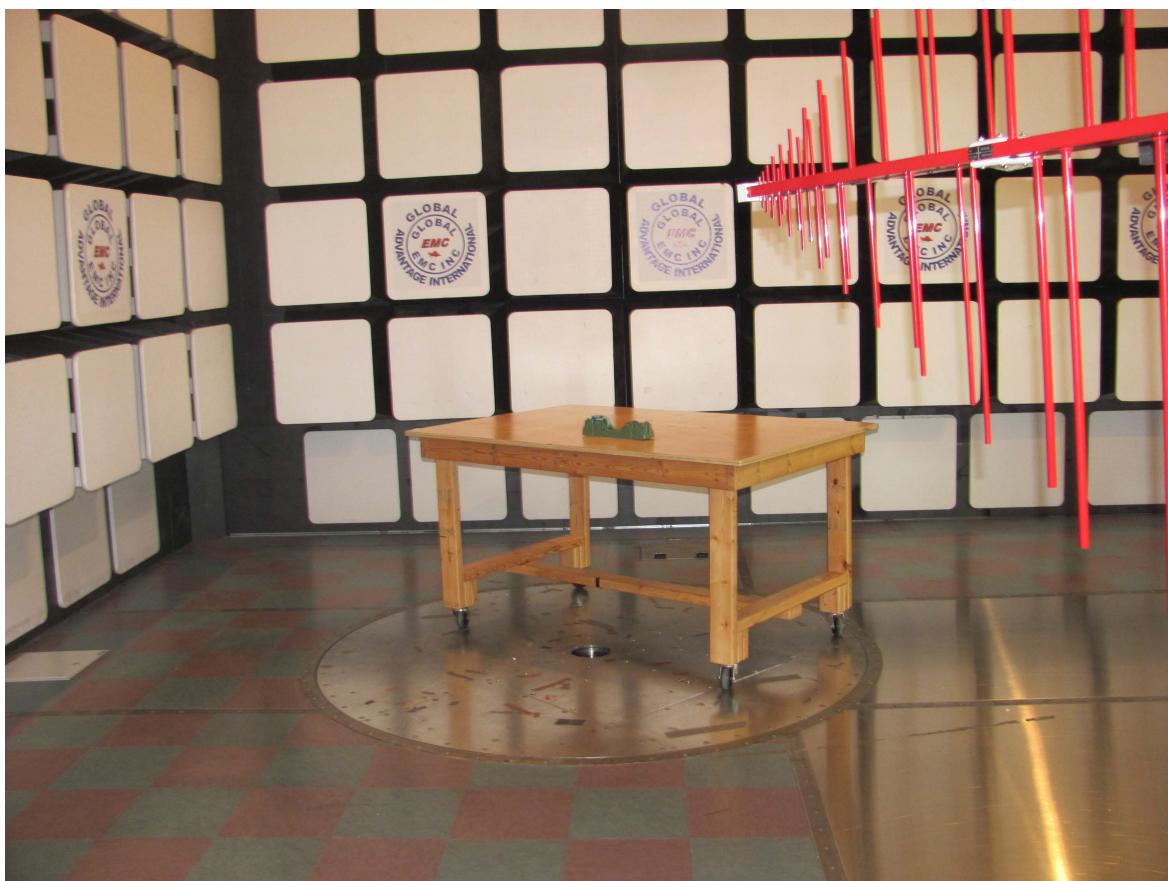
Illustration 2: Radiated emission setup - photo 2
