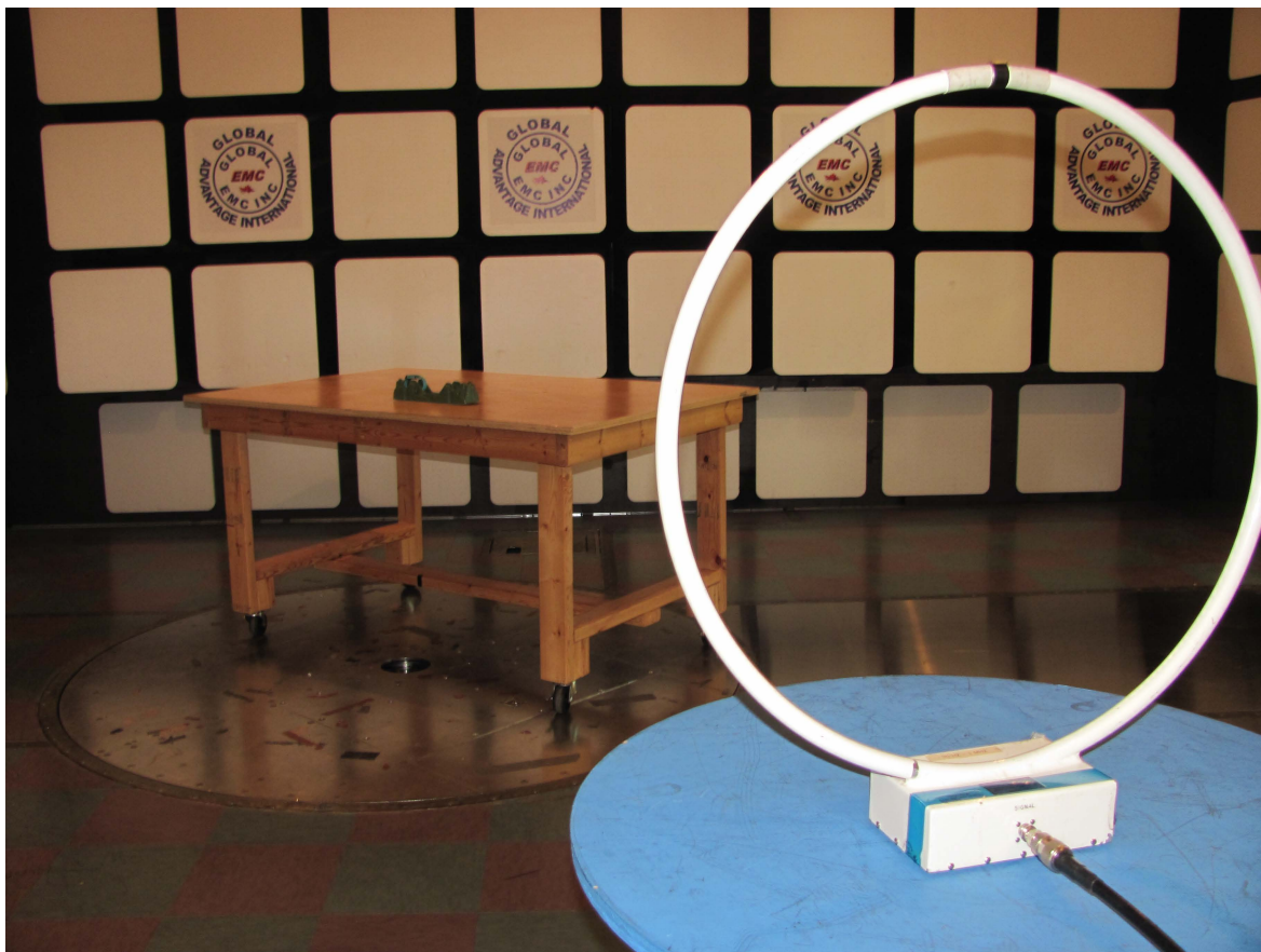
Illustration 1: Radiated emission setup – photo 1
