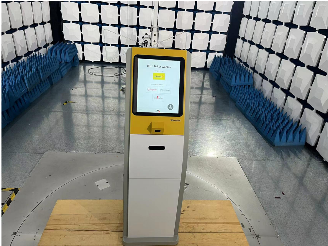
Blow 1GHz for radiated emission test setup
