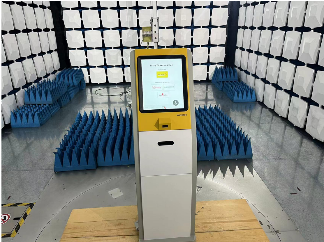
Above 1GHz for radiated emission test setup
