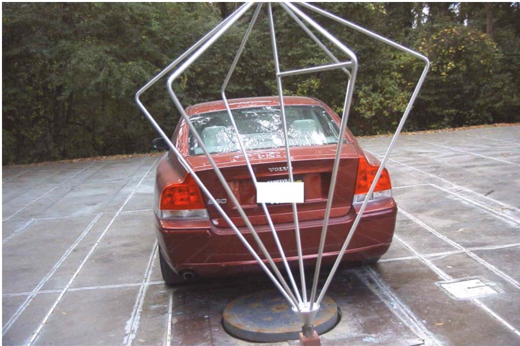
Lowest Margin for ST3/ST4 radio in 2005 Volvo S60 is at 180 degrees
