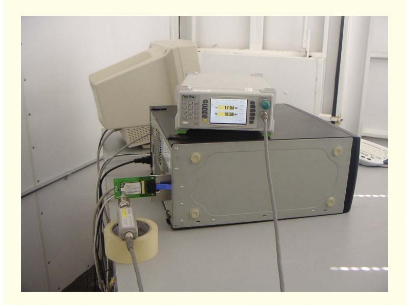
Maximum Peak Output Power Measurement Setup
