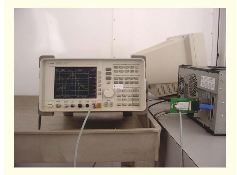
Conducted Emissions at Antenna Terminal Setup
