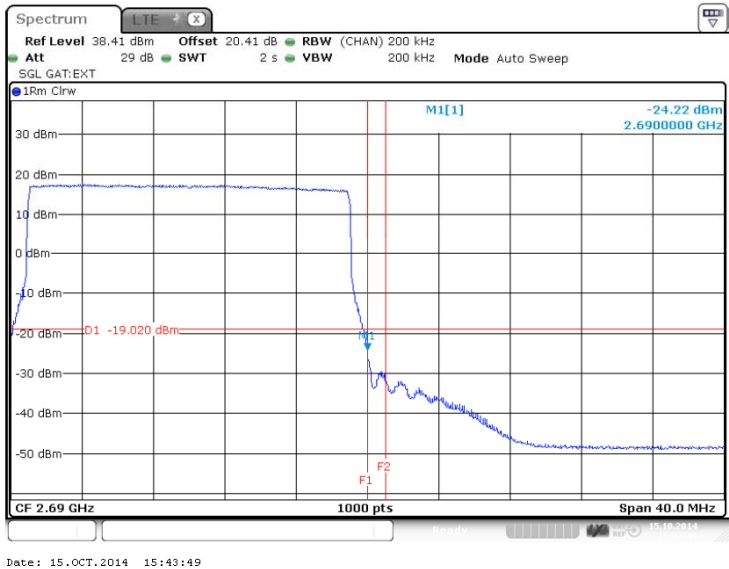
Figure 216 Spurious Emissions (Upper Band Edge) – QPSK (2680.0 MHz) (20MHz Channel BW)
