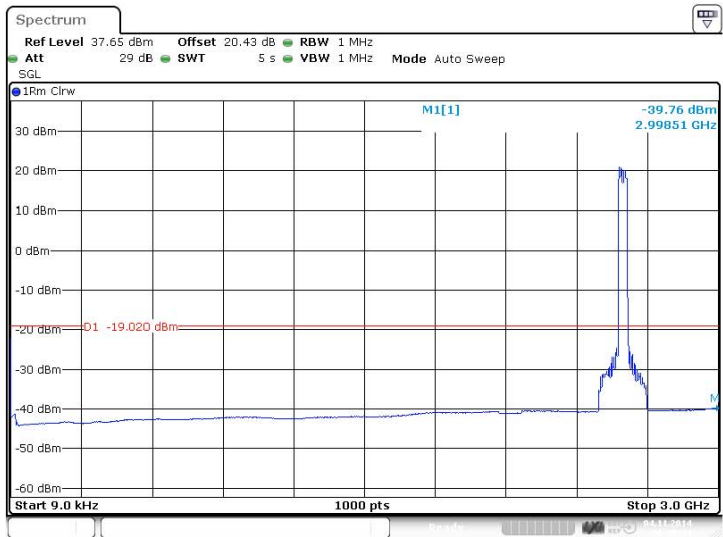
Figure 249 Spurious Emissions (9kHz – 3GHz) – 64QAM (2583.0/2603.0 MHz) (20MHz Channel BW)
