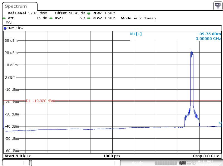
Figure 245 Spurious Emissions (9kHz – 3GHz) – 16QAM (2583.0/2603.0 MHz) (20MHz Channel BW)
