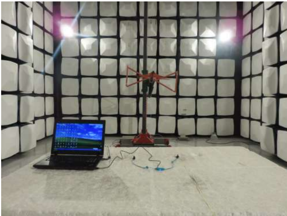
FCC RADIATED EMISSION TEST SETUP
