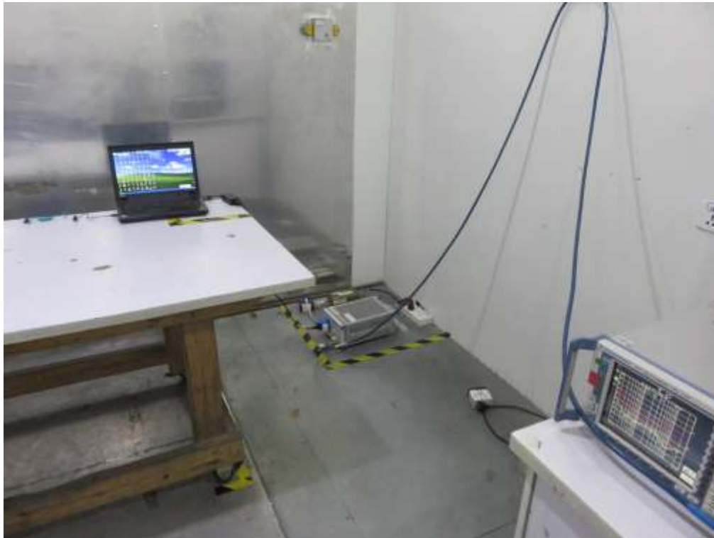
FCC RADIATED EMISSION TEST SETUP
