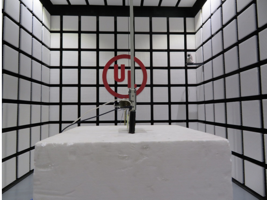
MEASUREMENT POSITION Y axis For 2G3GLTE Testing
