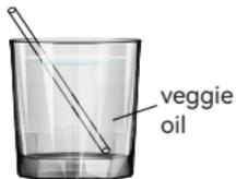
3.2 Put the head of hose into hot water for 10s or Put a little veggie oil on the end of the hose before connecting
