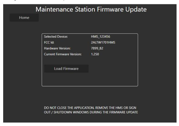
This label is shown on the monitor running the Hawk Maintenance Utility. The Hawk Maintenance Utility is connected to the hawk Maintenance Station via a USB cable
