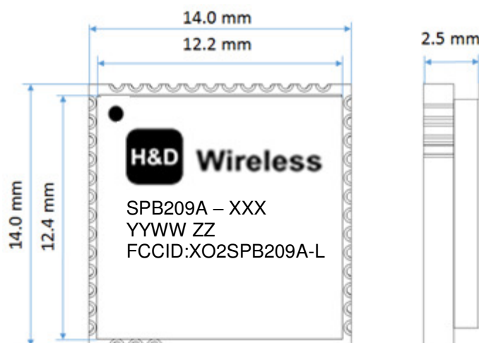
Figure 6.1: Mechanical drawing, equivalent to a 41 pin Quad Flat No-Lead (QFN) package.
