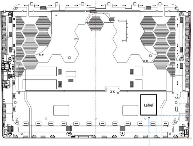
WLAN label is sticked on the core side of D cover.
