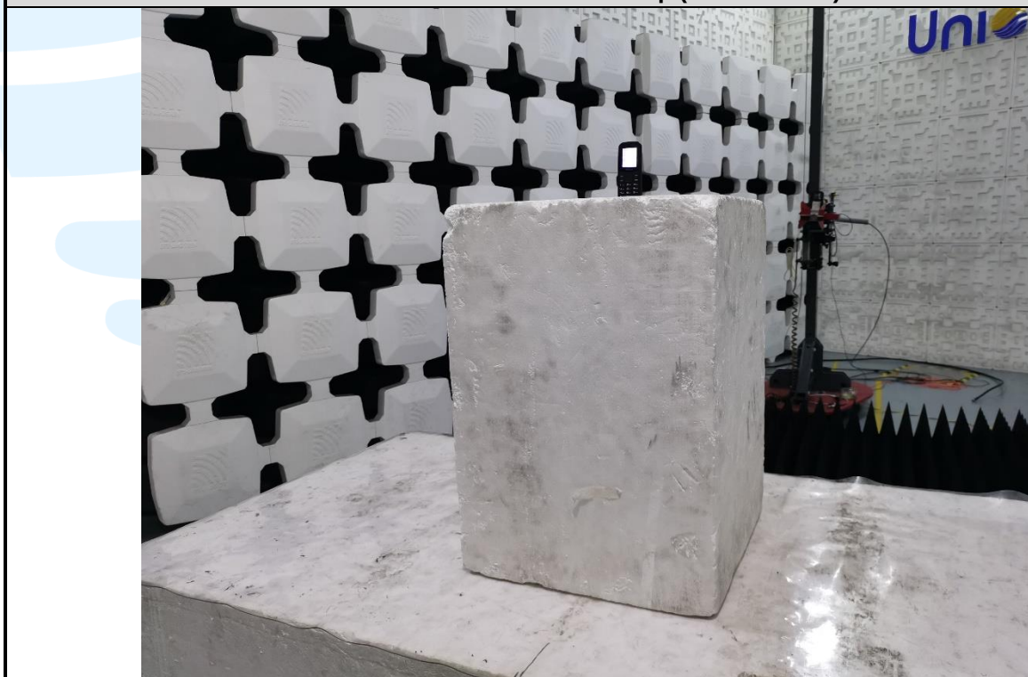
Radiated emission Test Setup (Above 1 GHz)
