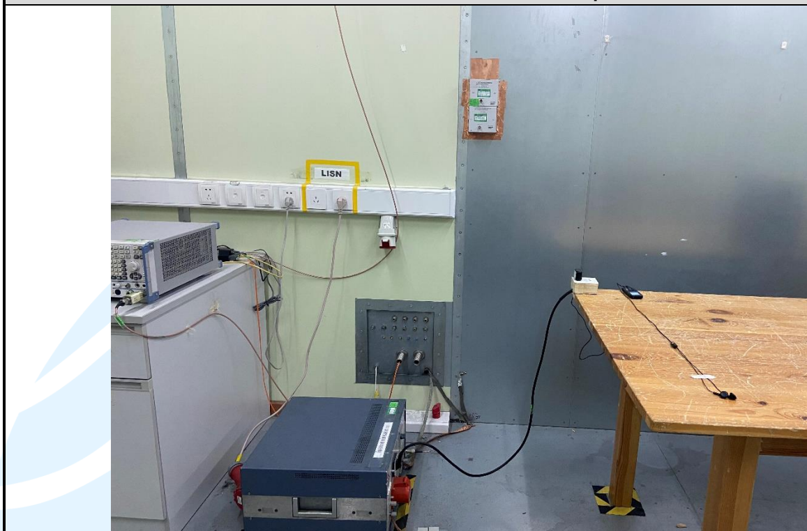
Conducted Emission Test Setup
