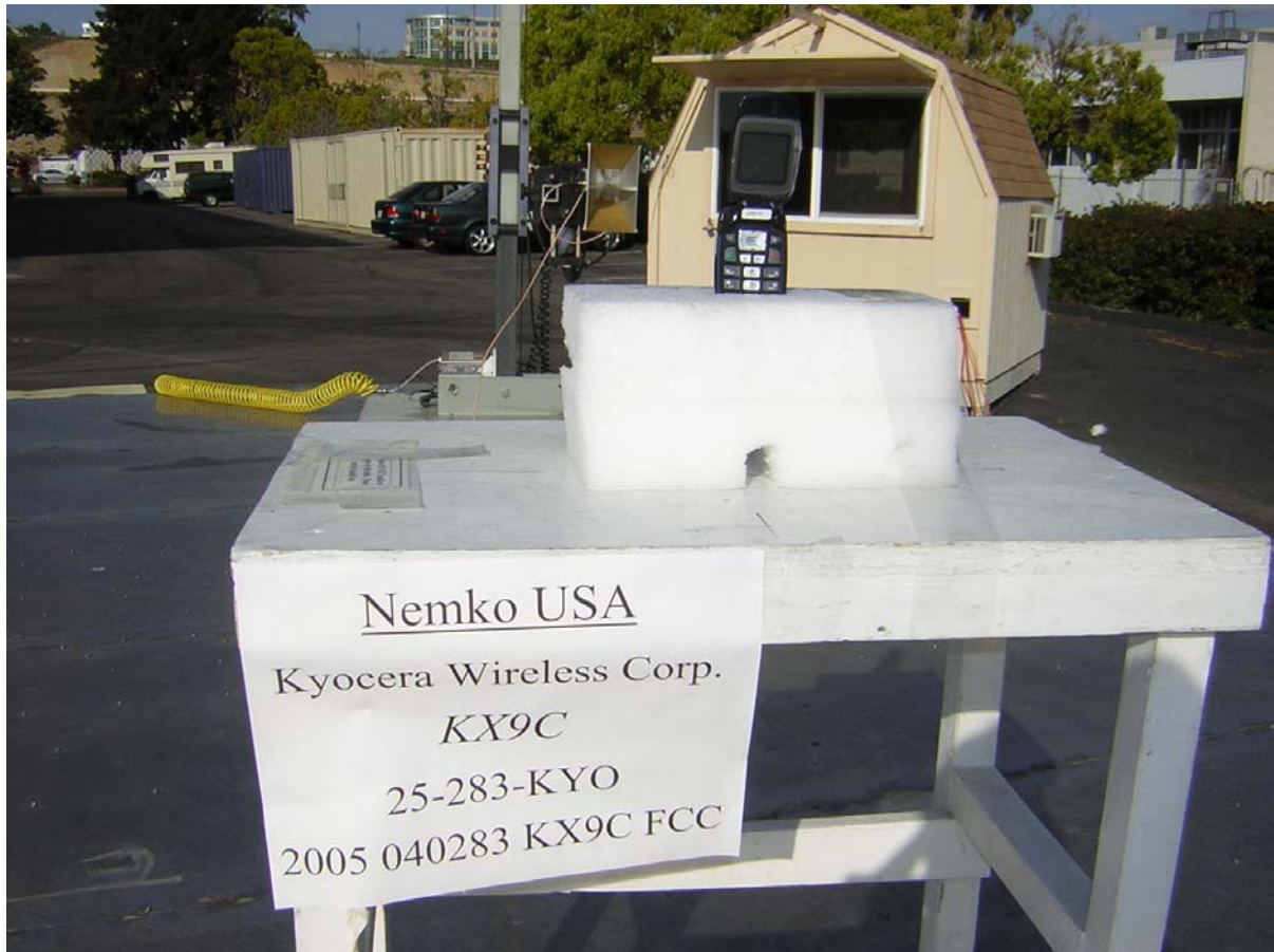
Photograph 2. FCC, Part 22/24 KX9C Test Configuration
