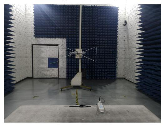
RADIATED EMISSION TEST SETUP ABOVE 1GHZ
