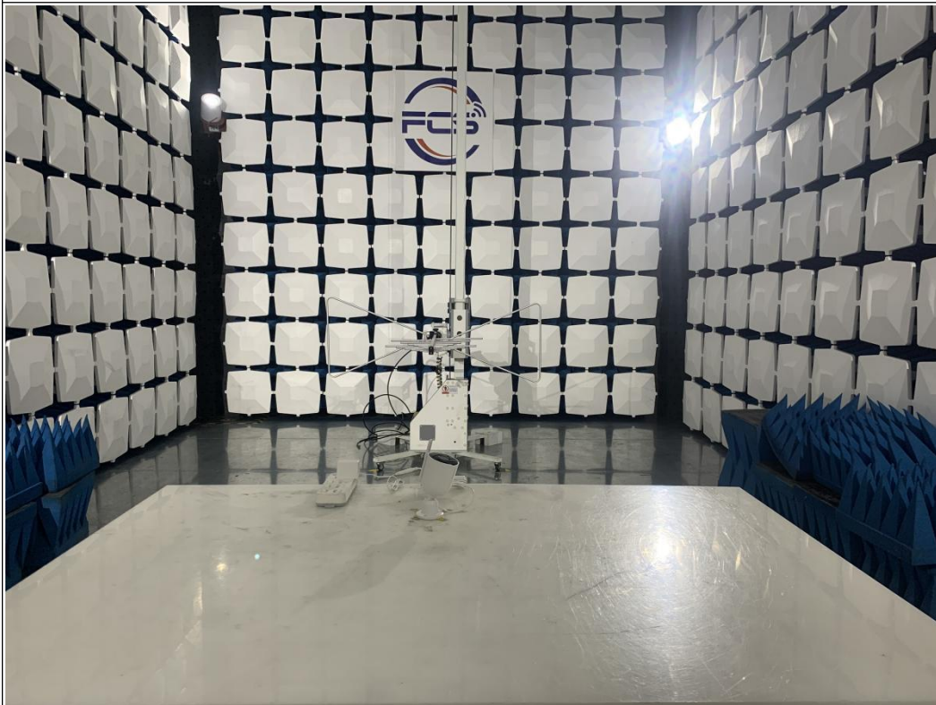
Above 1GHz for radiated emission test setup
