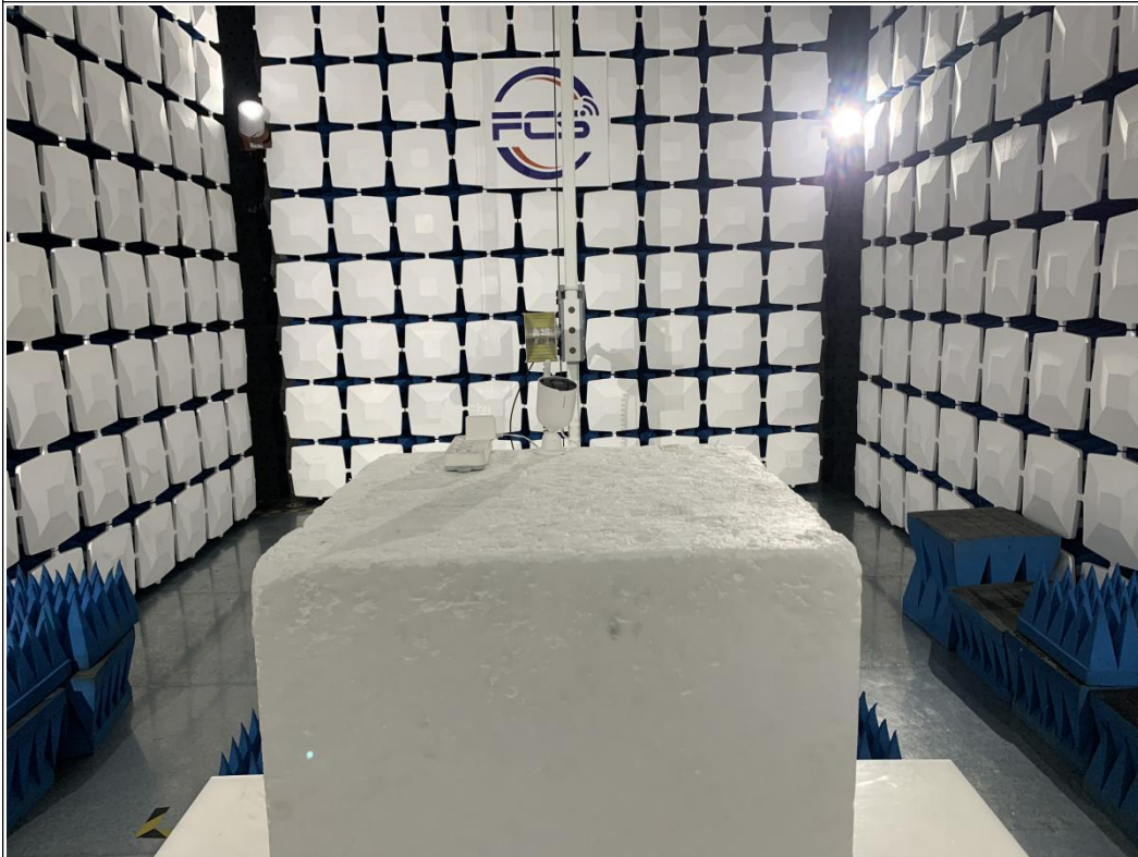
Above 1GHz for radiated emission test setup
