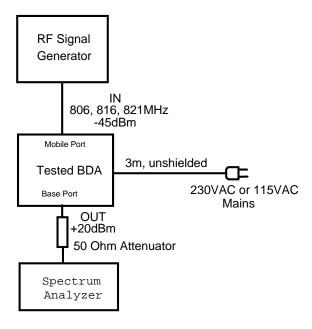
The tested equipment was conditioned with typical modulating signals to produce the worst case (i.e. the widest) bandwidth. In the case of MW-CBDA-ESMR-1W60 BDA 64kbits Per Second Pseudo-Random Digital Modulation was used.
