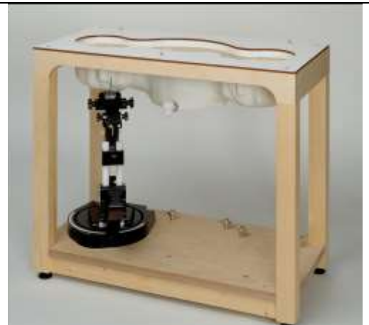
Fig. 8.7 Photo of SAM Twin Phantom
