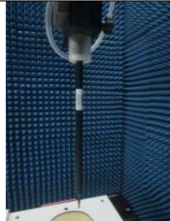
Fig. 8.2 Photo of E-Field Probe
