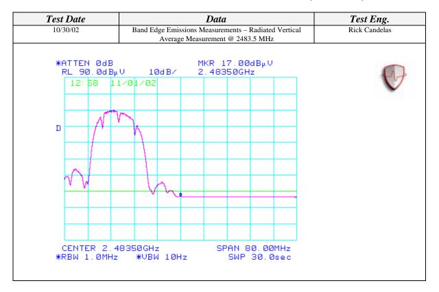
With the Ethertronics Dual Band Antenna
