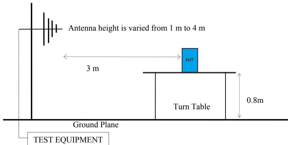
6.1.3. Fully Anechoic Chamber (3m) Setup Diagram for above 1GHz
