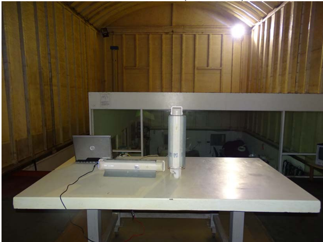
Back View of Radiated Test (Sector Antenna)
