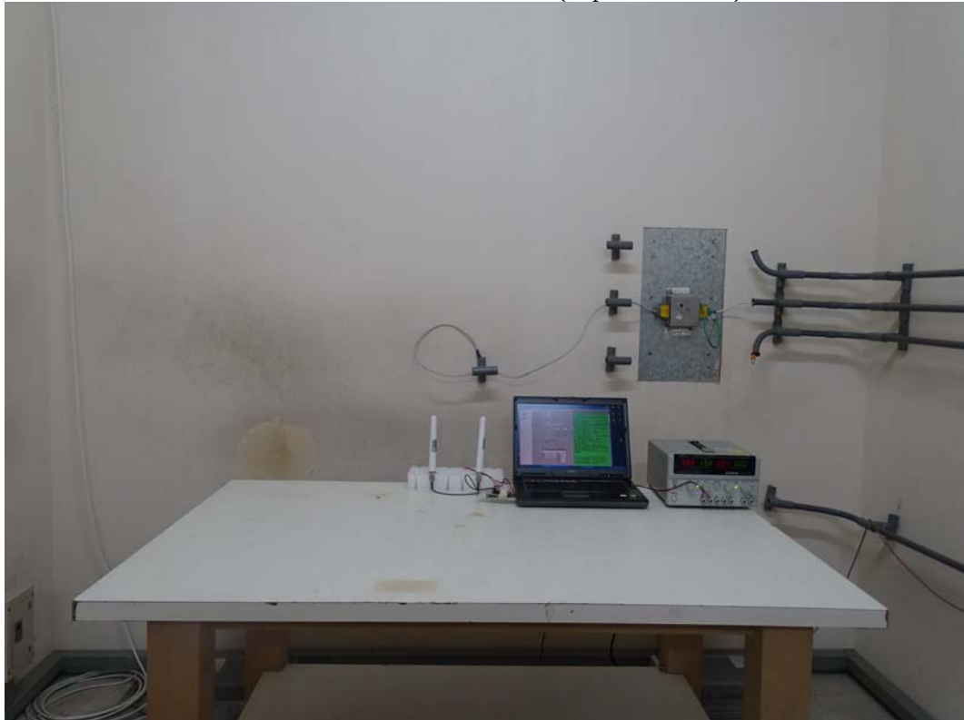
Front View of Conducted Test (Dipole Antenna)
