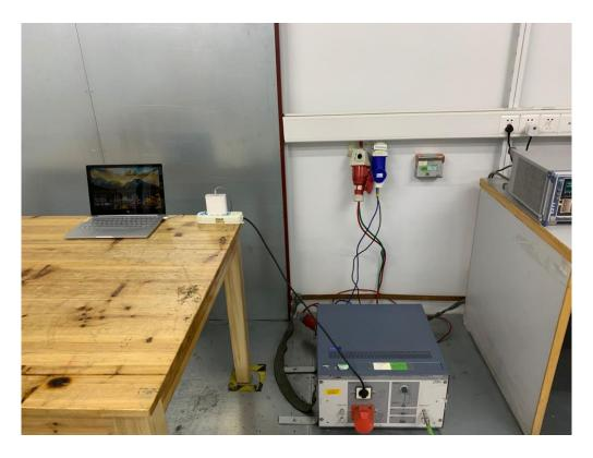
RADIATED EMISSION TEST SETUP BELOW 1GHZ
