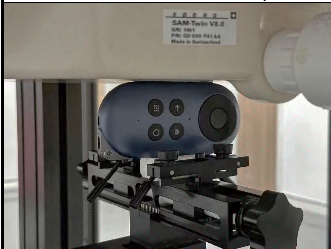
Left Side of EUT with 0 cm Gap
