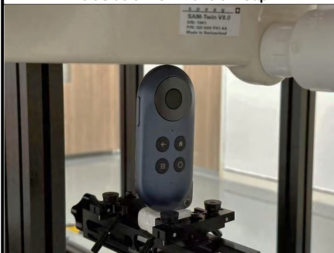
Top Side of EUT with 0 cm Gap
