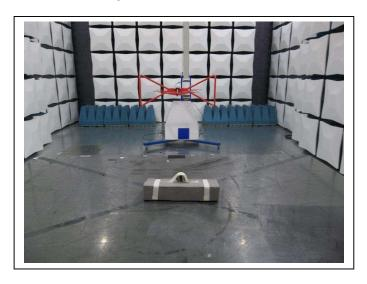
Radiated Spurious, Less Than 30 MHz
