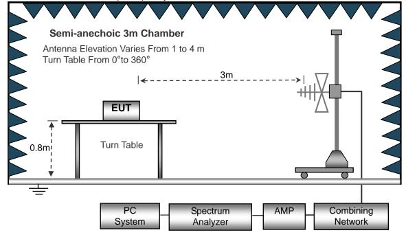
(C) Radiated Emission Test-Up Frequency Above 1GHz
