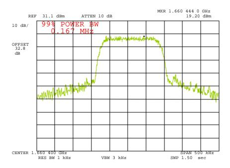
Power: Modulation: HIGH 16QAM, 151.2kHz Symbol Rate (20/5ms) 99% Power Bandwidth
