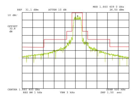
Power: Modulation: HIGH 16QAM, 33.6kHz Symbol Rate (20/5ms) 42K0G1D
