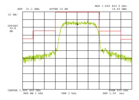
Power: Modulation: HIGH QPSK, 151.2kHz Symbol Rate (20/5ms) 200KD1W
