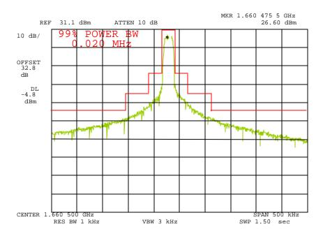
Power: Modulation: HIGH QPSK, 16.8kHz Symbol Rate (5ms) 99% Power Bandwidth
