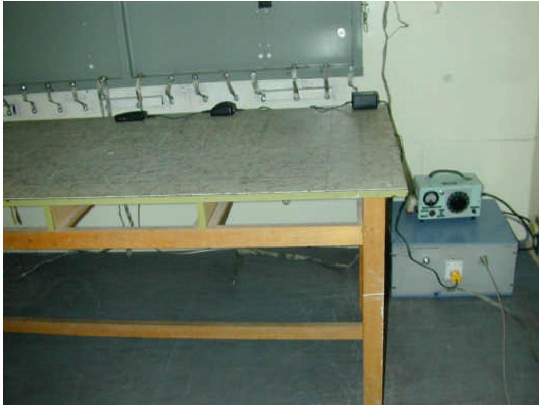
Photograph 4.1.1 Conducted emission measurements test setup
