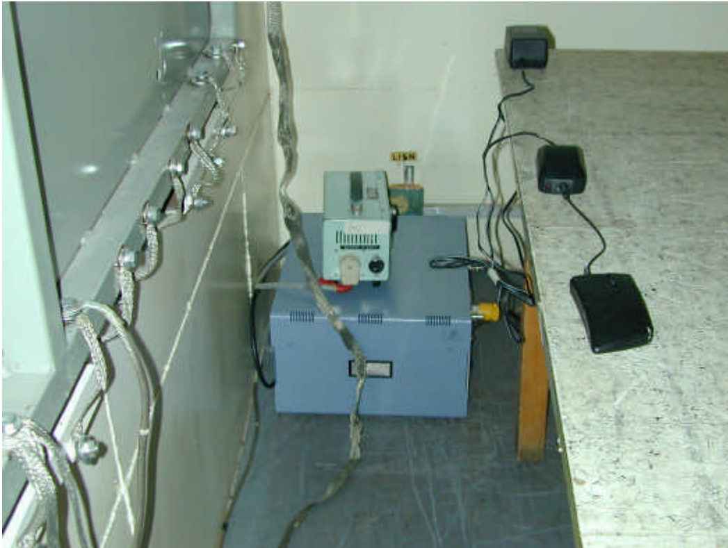
Photograph 4.1.2 Conducted emission measurements test setup
