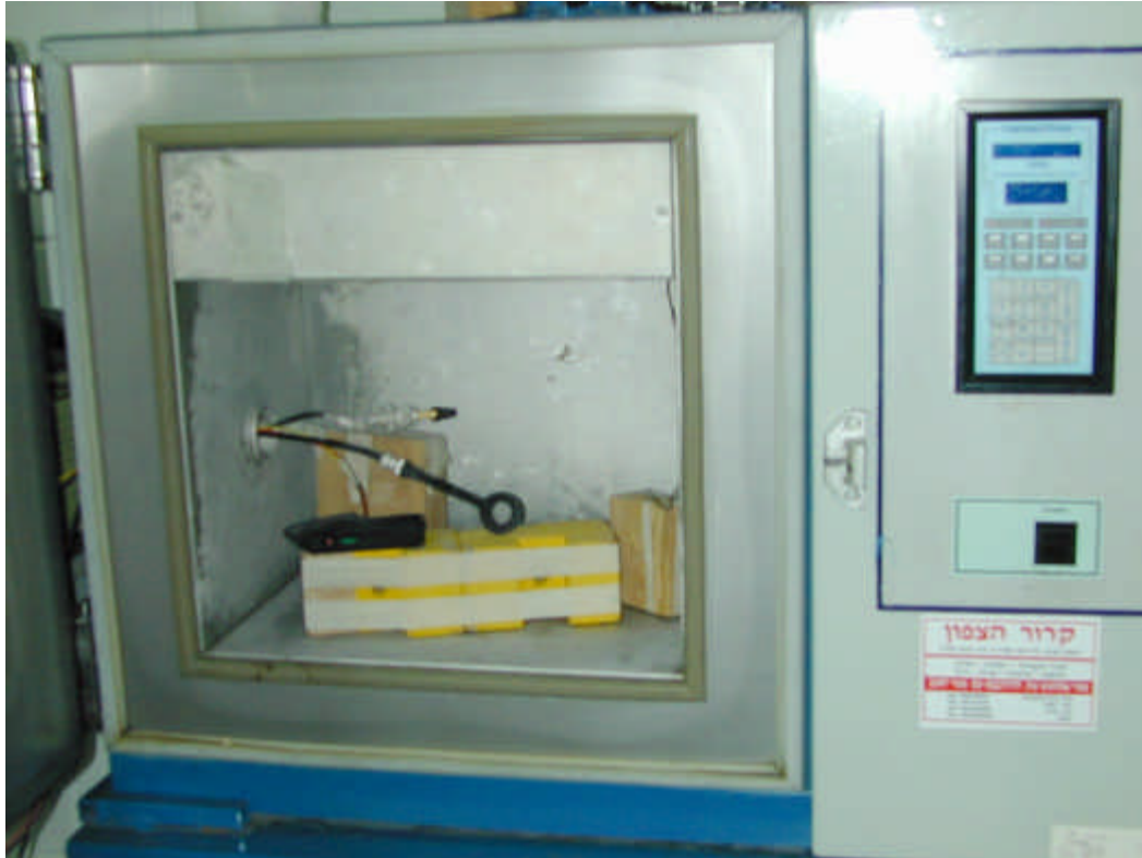
Photograph 4.6.1 Frequency stability test setup
